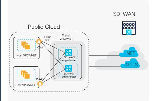
Each Cisco SD-WAN edge virtual router in the transit VPC builds two site-tosite IPsec tunnels (for redundancy, not for active/active paths) to the virtual private gateway (VGW) in the host VPC. There are two Cisco SD-WAN edge routers in the transit VPC, so the total number of IPsec tunnels in transit VPC is four.
