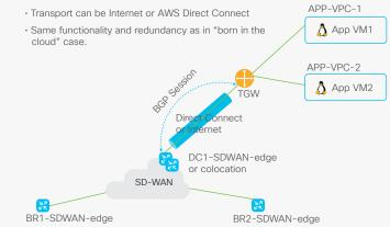
The same redundancy principle from Cloud OnRamp is used here: each SD-WAN edge router will establish two IPSec tunnels to TGW and run one BGP session per IPSec tunnel. So, there will be four IPSec tunnels and four BGP sessions in total between two WAN edges and TGW.
